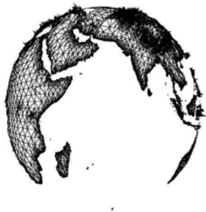
Fig 8 the delineation of global terrain based on hierarchical subdivision of the triangular meshes on ellipsoidal surface
